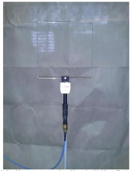
Figure 10. Quad Loop Antenna used to address the shielding effectiveness of the fabric, seen on the background.
